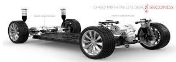
Figure 20 | Tesla model X chassis with two electrical motors
